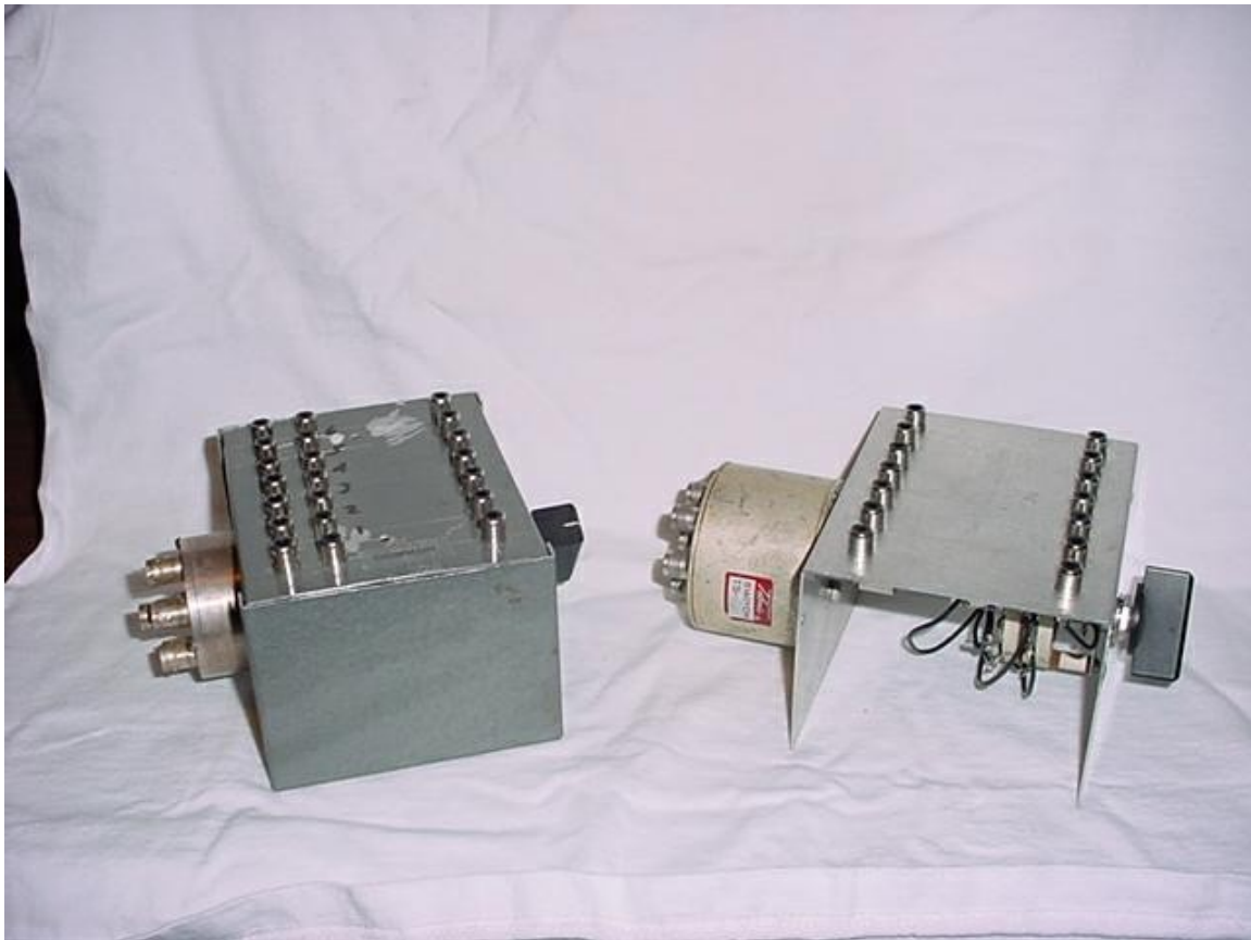
The rotary switch contacts added to rotary RF switches
